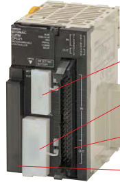
CPU Unit with Pulse I/O CJ1M-CPU21 160 I/O points, program capacity: 5 Ksteps, 16 built-in I/O points
